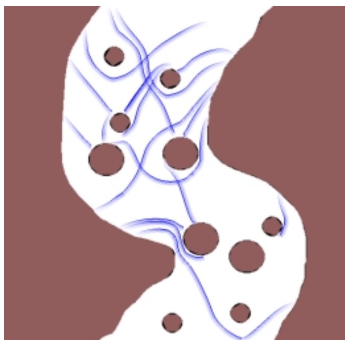
Fig. 11. Shockwaves built upstream and downstream obstacles.
