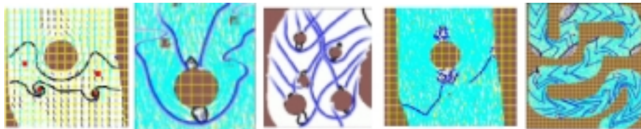
Fig. 9. Source and vortex perturbations make the brook quasi-stationary, showing evolving wave features (images are part of animations, which are available on our web site).
