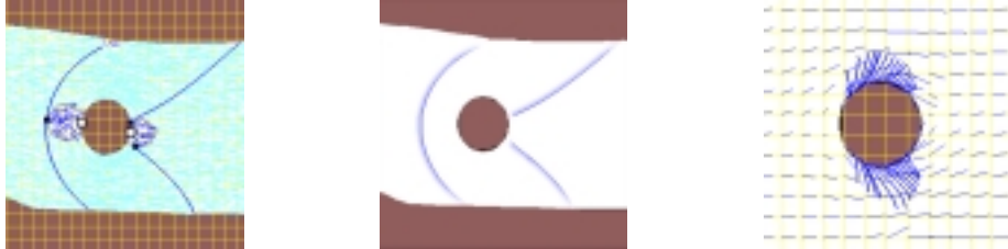
Fig. 5. Left: the various geometric constructions calculated in real-time by our simulator. The brook is designed by the user using a classical painter. The velocity field is solved on the 32 \times 32 grid (the flow is coming from the left; the light grey vectors correspond to supercritical flow, the dark grey to subcritical areas). The stop points are figured (the 2 white squares). The curves iso_{F_r=1} are traced in black. The starting locations of shockwaves found on the curves are marked as black squares. The upstream and downstream shockwaves (corresponding to four Froude lines) are shown in dark. Middle: the visible features obtained (i.e., the shockwaves and their associated ripples). Right: ripples along the sides.
