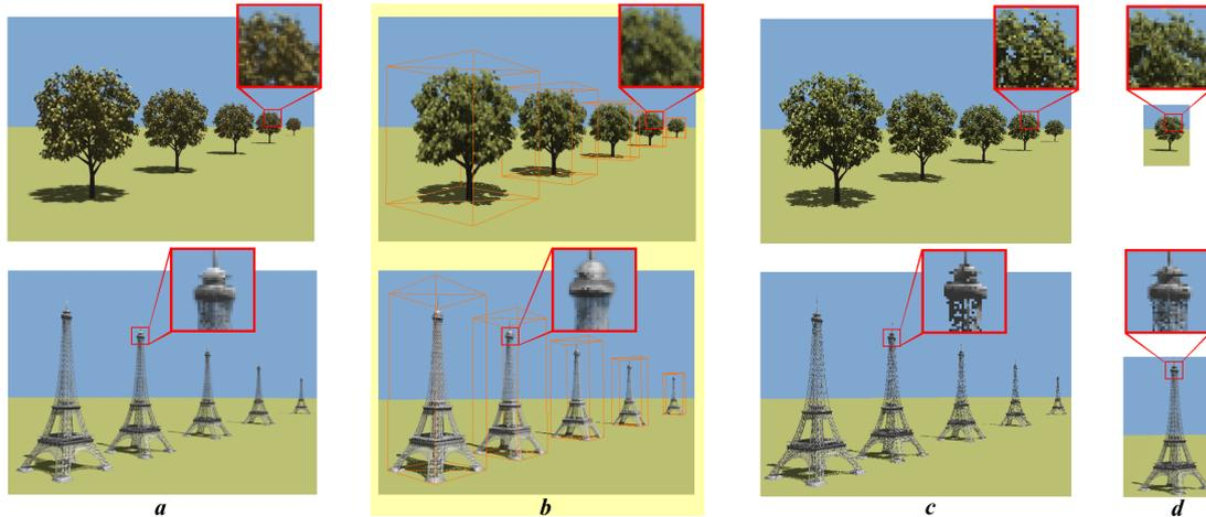
**Figure 7:** Comparison. Column **a**: Reference images (polygonal models rendered by 3DSMax). **b**: Our method ( $256^3$  and  $128 \times 128 \times 256$  MIP-mapped volumes). **c**: Real-time rendering of the polygonal models (200000 and 22600 faces). **d**: Same as **c** with FSAA $\times 8$  enabled.
