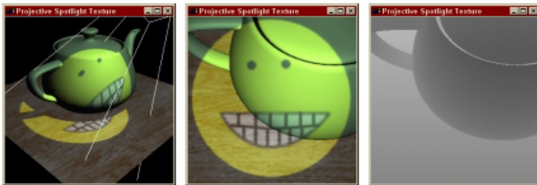
Figure 11 - Scene rendered from camera (left), and light (middle). Depth buffer from the light's view (right) 14
