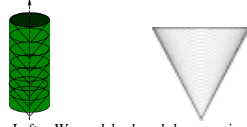
Figure 6: Left : We model a bough by a semi-opaque volumetric cylinder, which opacity is anisotropic in order to reproduce the variation of the number of intersection between a ray and the sub cones. Right : Intersection of the plane P_r with one cone. We approximate the hyperbolas by their asymptotes.
